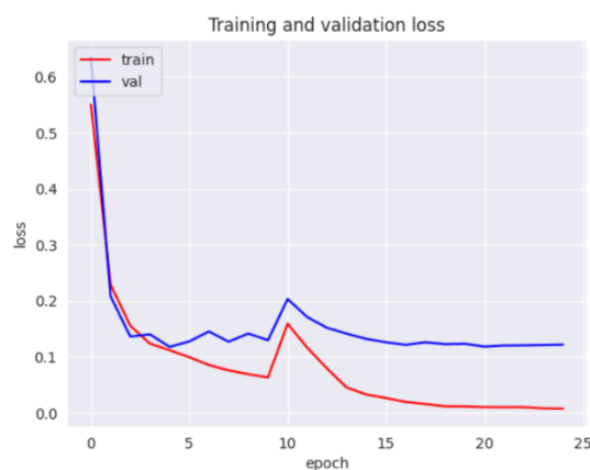
Figure 9. Loss progression of the ResNet50 model
